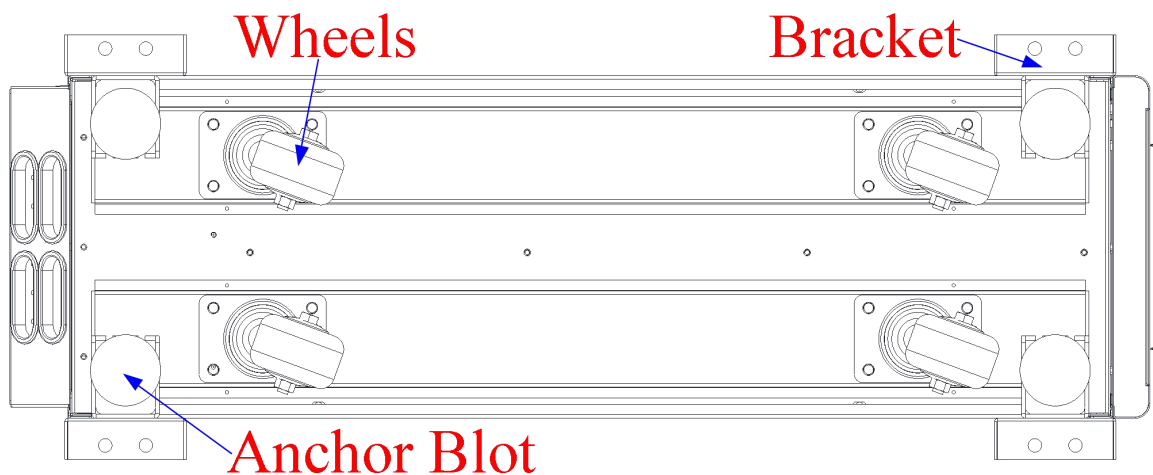
Fig.3-1 Supporting structure (Bottom view)
