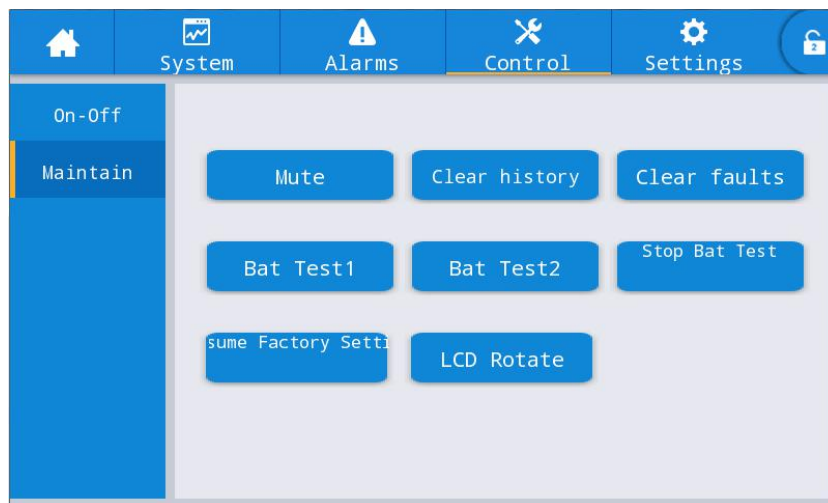
Fig. 5-4 Battery maintenance page
